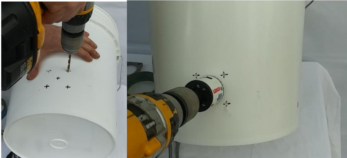
Figure 5 Drill pilot and center holes.
